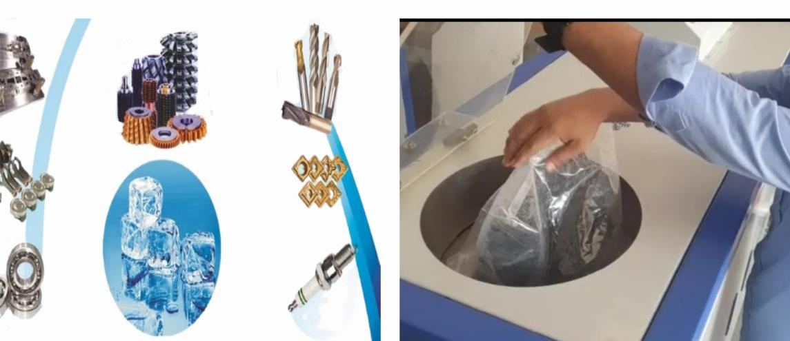
We offer job work assistance requiring deflasjing either in cryogenic and/or spin trim deflashing machine depending upon part geometry, volume and flash condition etc.
